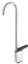
Model 5551 Push lever operated, self-closing, polished chrome-plated brass, deck-mounted, gooseneck cold water glass-filler faucet.
